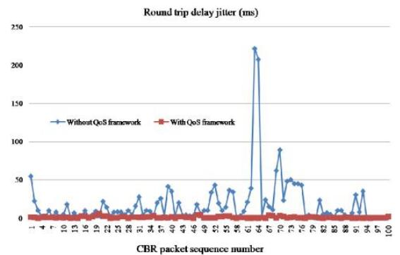
Round trip delay jitter of CBR packet
